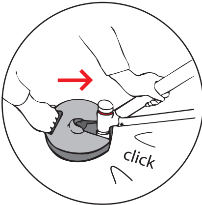
4. Install the four weighted plates (one on each corner) and listen for the "click"
