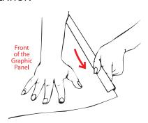
5. Slide the profile onto the top of the new graphic panel.
