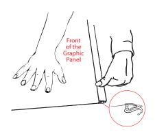
6. Press down on the profile to lock it onto the new graphic.
