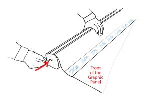
2. Pull the graphic until the lead sheet is exposed and slide the pin into the hole on the side of the base. Please note: if the locking pin does not slide in all the way. It may be necessary to slowly pull out the graphic or retract it slightly until the pin slides into place. If you do not have the pin, you can use a strong paper clip or a small allen wrench.
