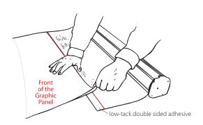
7. In some instances, their may be enough adhesive on the lead sheet to mount the new graphic. If not, we highly recommend using our double sided lead sheet tape (article number: 69002) and reapplying it above the red line. Attach the new graphic (image up) and position the bottom of the graphic panel along the red line.
