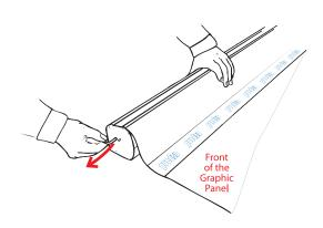
9. Grip the image and base firmly with the left hand . Remove the locking pin with the right hand.
