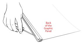
4. Using a flat blade screwdriver (or similar tool) open the profile and remove it from the old graphic panel.
