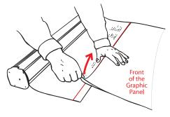
3. Remove the securing tape and pull the graphic off of the white lead sheet. Cutting the lead sheet will void the warranty.
