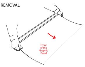
1. Pull the graphic panel out of the unit. Working on a clean surface such as a work table and using two people will make this easier. One person should securely hold the base and the other should pull out the graphic by the top profile.
