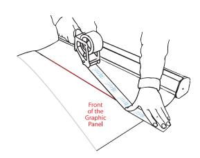
8. **IMPORTANT!** Apply packing tape over the joint to secure the graphic panel to the lead sheet. We highly recommend using the Expand Logo Tape (article number 69003) for this step. This tape is extremely durable and since it is much easier to remove than standard packing tape, it will make your graphic switch out process much quicker.
