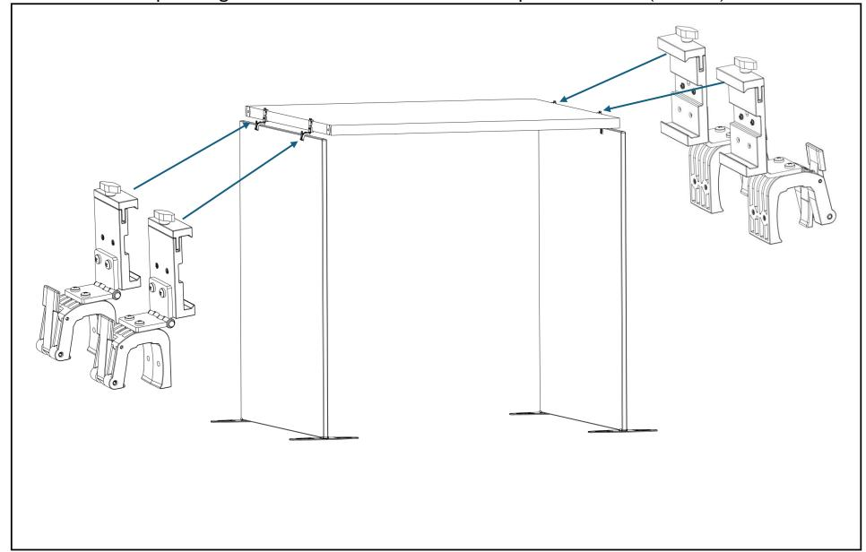
Expand LightBox roof with 2 EGF walls Set-up Instruction (A108-2)
